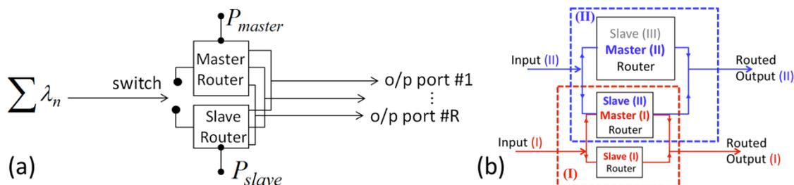
Fig.1. (a) Master-slave configuration for edge-routers; (b) Schematic of two successive generations (I) & (II) of master-slave configurations.
