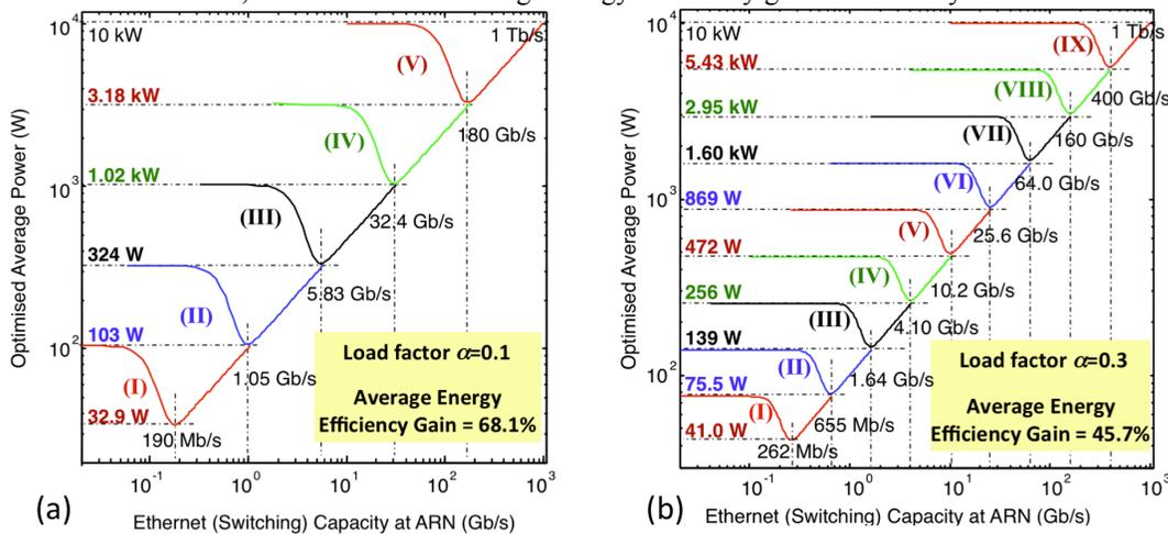
Fig.3. Upgrade trajectories from 1Gb/s→1Tb/s: (a) 5 generations for  $\alpha=0.1$ , efficiency gain  $\eta=68.1\%$ ; (b) 9 generations for  $\alpha=0.3$ , and  $\eta=45.7\%$ .
