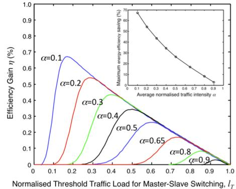
Fig. 2. Efficiency gain curves for different  $\alpha$  values as a function of varying normalised threshold traffic load  $l_T$
